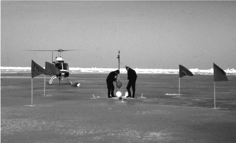
Figure 1.4 Deployment of a corner reflector mast for deformation studies by a laser geodimeter, in the Baltic Sea in April 1978. A system with several reflector sites allows accurate monitoring of sea ice kinematics in a 5 km scale array.
