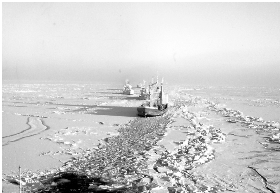
Figure 8.7 Convoy of ships assisted by an icebreaker in the Baltic Sea. Ice dynamics determines the length of a convoy.
