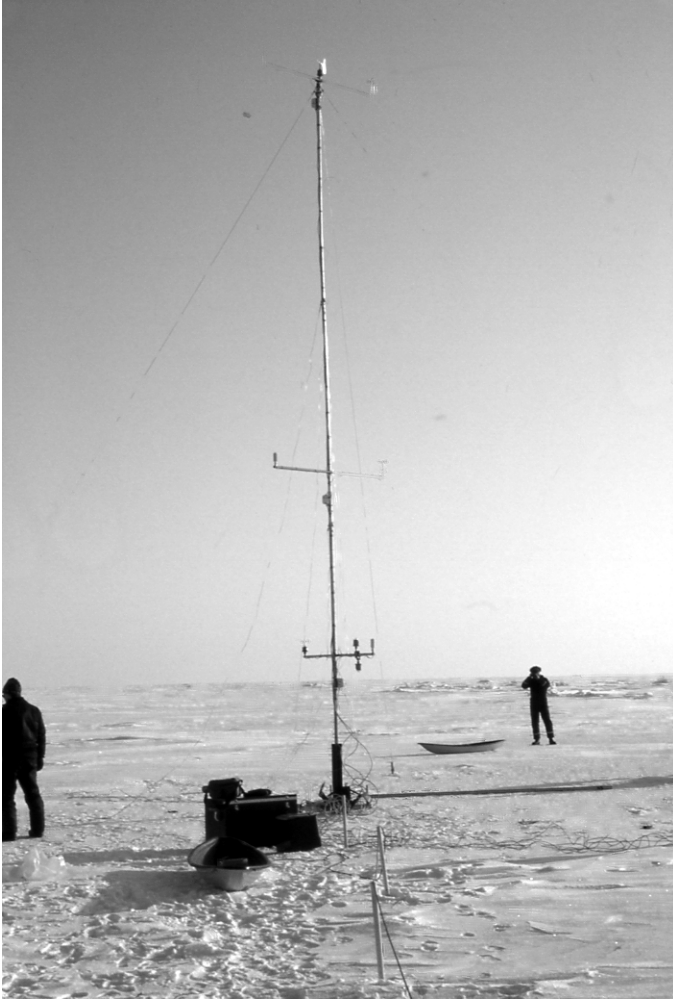
Figure 5.6 A mast (height 10 m) for atmospheric surface layer measurements. Velocity, temperature, and humidity are measured at several altitudes to determine the fluxes using the so-called profile method.
