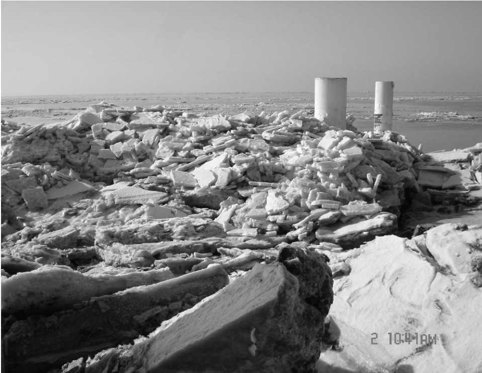
Figure 4.13 Ice ride-up on shore in the Bohai Sea. The diameter of the cylinders is about 1 m. In the front sediment-enriched ice floes are seen.
