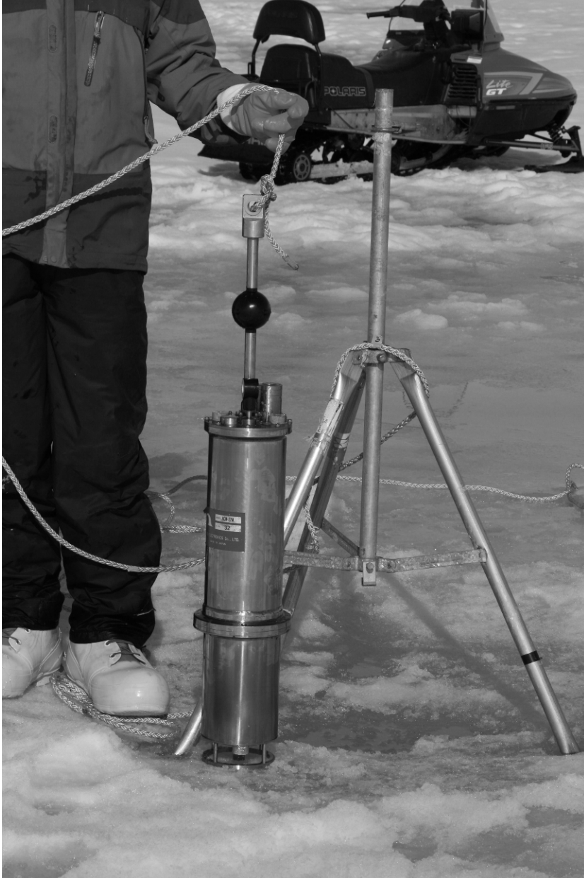
Figure 5.9 Current measurements by a three-dimensional electromagnetic current meter (Model ACM32M, Alec Electronics Co., Ltd., Japan). One person lowers the current meter through a drill hole and fixes it with a tripod at the depth of 1 m (as the reference level) below the ice bottom in the oceanic boundary layer.
