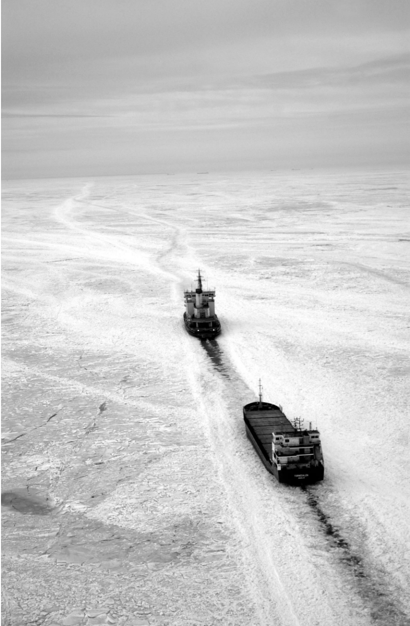
Figure 1.3 Icebreakers have extended navigation season in ice-covered seas since late 1800s. Their operation is sensitive to ice dynamics, due to ice pressure and thick deformed ice formations. Icebreaker Sisu assisting a cargo vessel in the Baltic Sea. Photograph by Mr. Riku Lumiaro, printed with permission.
