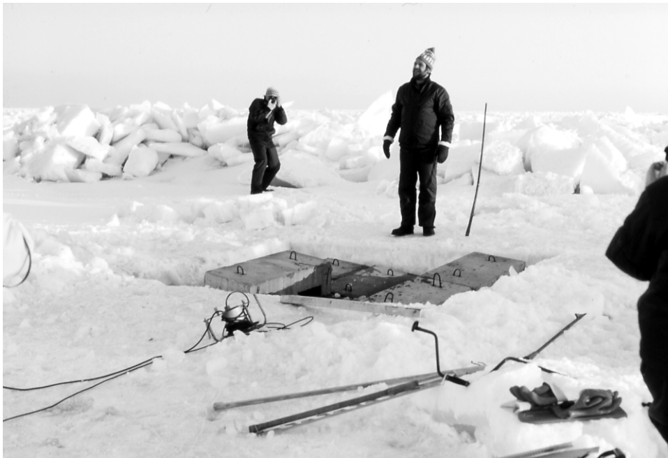
Figure 4.6 Field experiment into the strength of sea ice ridges in the Baltic Sea, winter 1987. The ridge keel is loaded with weights to examine the Mohr–Coulomb model.
