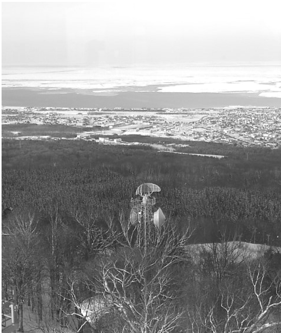
Figure 3.5 Mombetsu X-band ice radar antenna on top of Mt Oyama (300 m) monitoring the sea ice of the Sea of Okhotsk.
