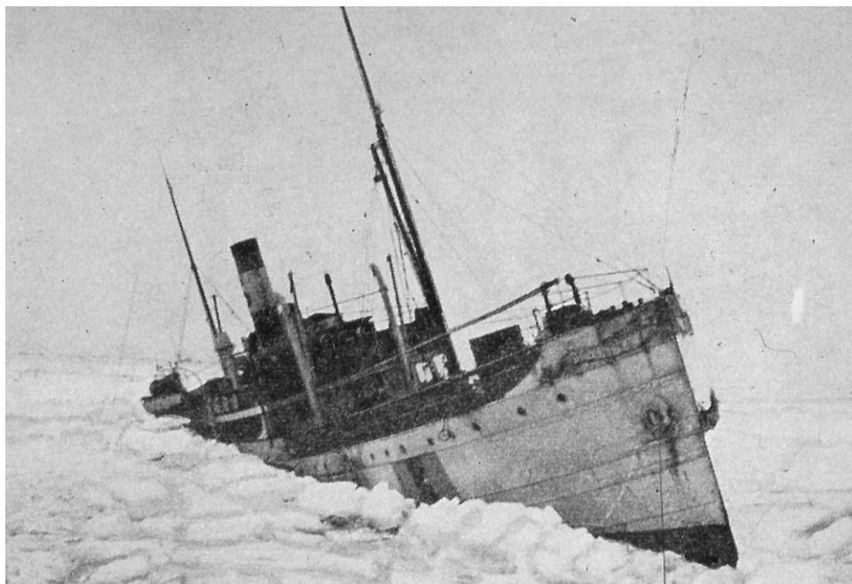
Figure 4.12 Ice pressure has captured one ship in the Baltic Sea. The strength of the ship is known but it is very difficult to predict local scale ice forcing from geophysical scale sea ice dynamics.
