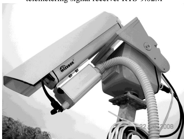
Fig. 3.4.6. Thermal case with cleaner and washer, fixed on the support rotating device
