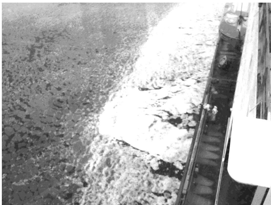
Fig. 3.5.6. Example of icebreaker hull “Kapitan Dranitsyn” covering with ice in the northern Laptev Sea (coordinates 79^{\circ} 15' \text{ N} , 125^{\circ} 47' \text{ E} ) on the 2 nd of September, 2003 with nilas. Top view, along the board. Intensive white part along left bow of icebreaker – snow-ice pillow.
