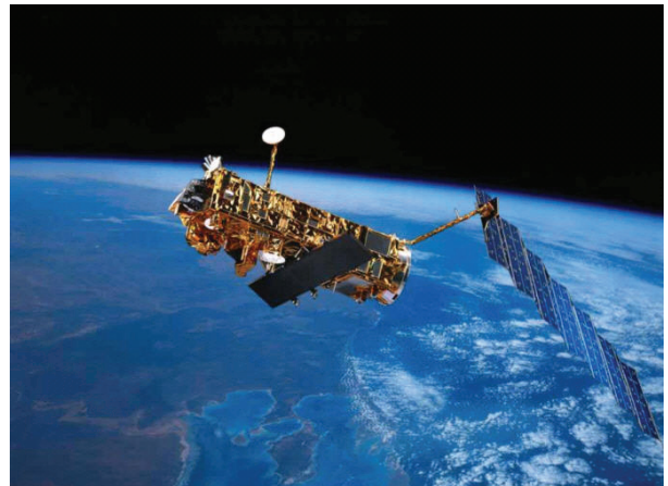
The SAR sensors on the European Space Agency's ENVISAT satellite and the Canadian Space Agency's RADARSAT satellite are excellent tools for observing ice.
